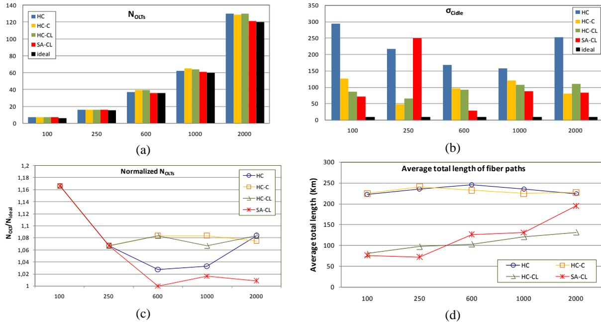
Figure 2 (a) number of PON segments/OLTs per scenario (b) std. deviation ( $\sigma$ ) of spare capacity per segment/OLT, (c) normalized figure of OLTs over the ideal minimum (d) average total length of fiber paths
