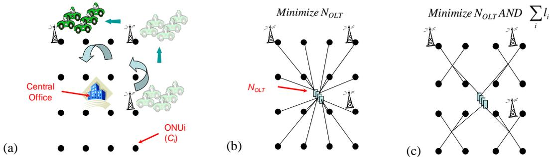
Figure 1 (a) spatial distribution of fixed and mobile terminals (and potentially temporal distribution of capacity demand), (b) potential PON backhaul design serving capacity demand, (c) potential PON backhaul design optimizing total fiber path length
